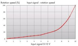
The input signal is directly proportional to the efficacy of the rotor, which implies that input signal and rotation speed are as per the adjacent diagram.
